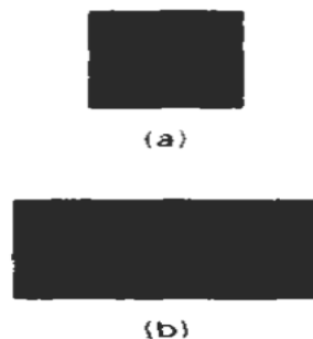
Figure 5-6 Turning a square (a) into a rectangle (b) with scaling factors s_x = 2 and s_y = 1 .
